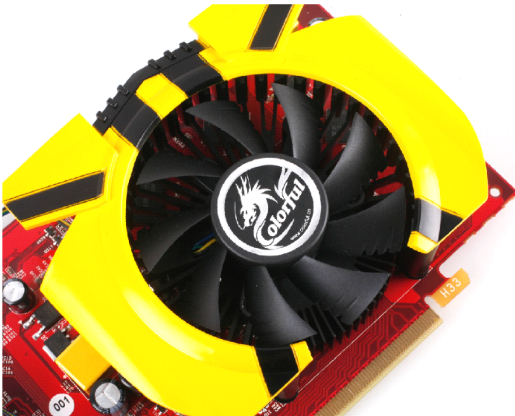
Using BUMBLEBBE Cooler, with Air Guided Notches, Fan Cowl and Step Design
