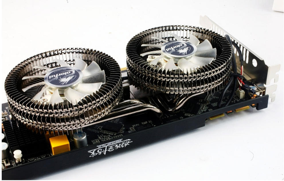
Dual-fan blade design, 4 pure copper heat-pipes, pure copper base
