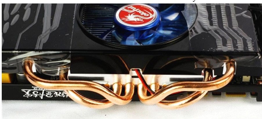
4 pure copper heat pipes
