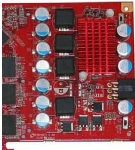
3+1 phases Power Supply System: Using high quality inductors and capacitors
