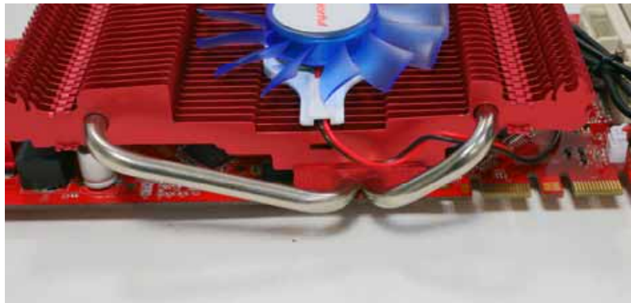
High efficiency fan with heat pipe
